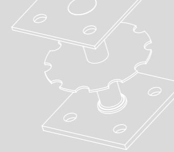
Chaplets designed for castings where **perfect pressure seal** is required, such as hydraulic castings, automotive castings, pumps, boilers, etc.
